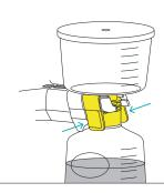
To detach the bottle, grasp the funnel and unscrew it, along with the yellow adapter, then lift it off the bottle.
