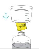
For vacuum filtration units (Sartolab® RF), unpack the sterile screw cap and securely close the bottle for storage.
