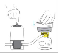
To end filtration, turn off the vacuum source and detach the tubing from the connector.
