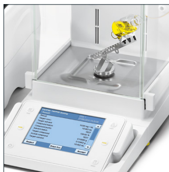
Step 4: Check the achieved results gravimetrically
