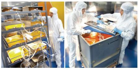
Figure 3. 2D-bags and 3D-bags for buffer storage, 2D-bags are installed on trays, 3D-bags are installed in palletanks.
