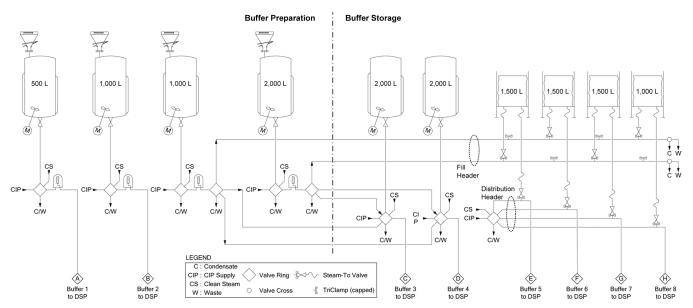
Figure 4. Process flow diagram for buffer preparation and buffer storage. Connecting points <A> to <H> refer to P&I-diagram in Figure 6.
