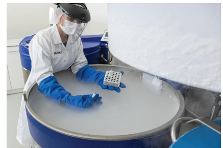
Photo 3: Setting up a master cell bank (MCB) by placing cell stocks in liquid nitrogen for long-term storage
