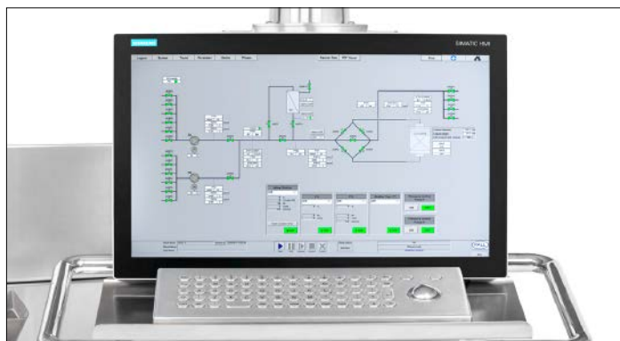
Figure 3: Fully Maneuverable Touchscreen Human Machine Interface (HMI)
